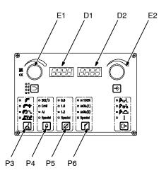
Set Synergic MIG welding process using P3 push button.
